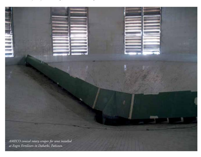
The ET scraper pivots a few degrees left and right at the summit of the stack. As soon as the rake chain leaves the stack, the pivoting action stops, the scraper arm is lowered to a few degrees and the pivoting action is resumed in the opposite direction.
